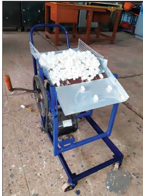
Fig. 15.5: Deflossing machine with cylinder and emery paper mounted on trolley with wheels
