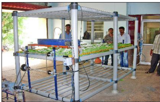
Fig. 16.2: Mechanized rearing beds for late-age silkworm rearing
