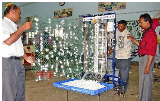
Fig. 16.1: Machine for harvesting cocoons from collapsible plastic mountages
