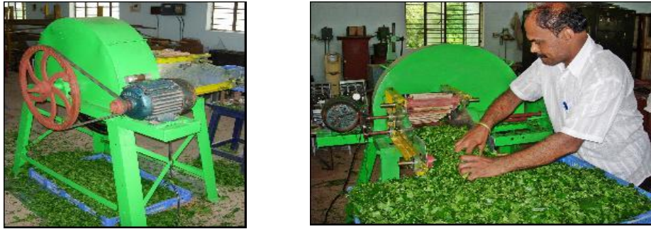
Fig. 16.4: High capacity mulberry leaf chopper for commercial chawki rearing centres
